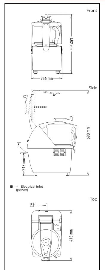
Electric Supply voltage: 200-240 V/1N ph/50/60 Hz Electrical power, max: 1.3 kW **Total Watts:** 1.3 kW Capacity: Performance (up to): 2.5 kg/Cycle **Capacity:** 5.5 litres Key Information: External dimensions, Width: 256 mm External dimensions, 415 mm Depth: External dimensions, Height: 482 mm **Shipping weight:** 23 kg
